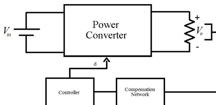
Figure 1: Simplified block scheme of a power converter
